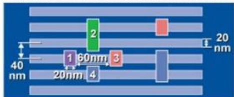
Final pattern requires 4 “cut” masks with Optical Litho, or 1 “cut” mask with EUV
