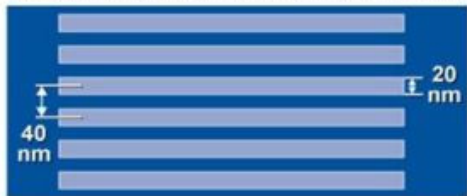
Final pattern requires 4 “cut” masks with Optical Litho, or 1 “cut” mask with EUV
