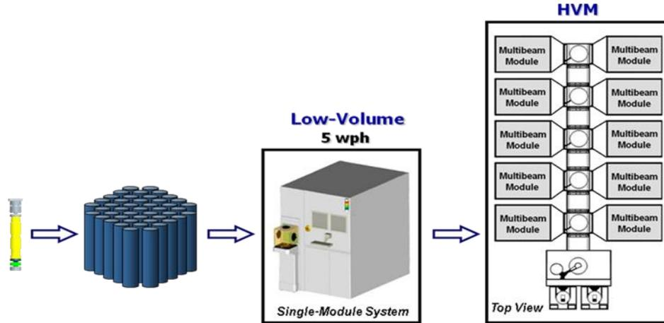
Figure 3. Multiple modules can be integrated in a cluster configuration for HVM.
